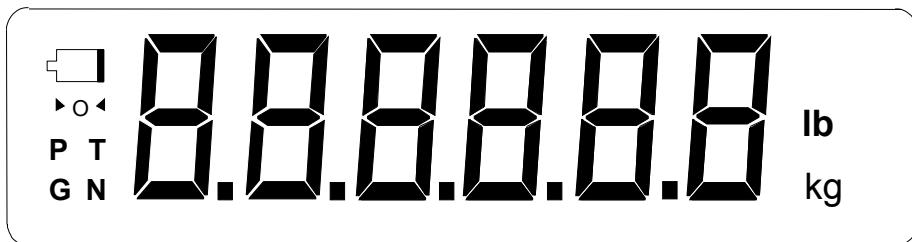
Figure 7-13 BB-1107 LCD Detail
